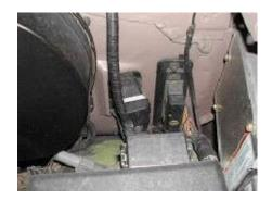
On the firewall by the driver's side fender well and to the right of the Main Wire Harness Bulk Head, you will find a connector plug with a bolt in the center, remove bolt (10mm head) and slide off the plug.
