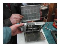
**<u>NOTE</u>**: There is a plastic spacer that supports the circuit board in the box. It is not attached and will be loose when you pull the box apart. **DO NOT LOSE THE PLASTIC SPACER**.
